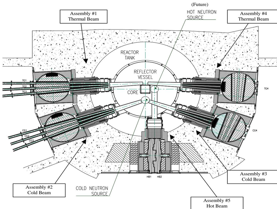
Fig. 2. Neutron beam arrangement.
